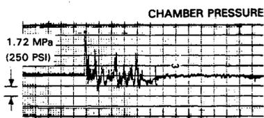
Fig. 15 Pressure trace exhibiting the damping characteristics of the FRT injector when perturbed with a 13.5-grain bomb.
