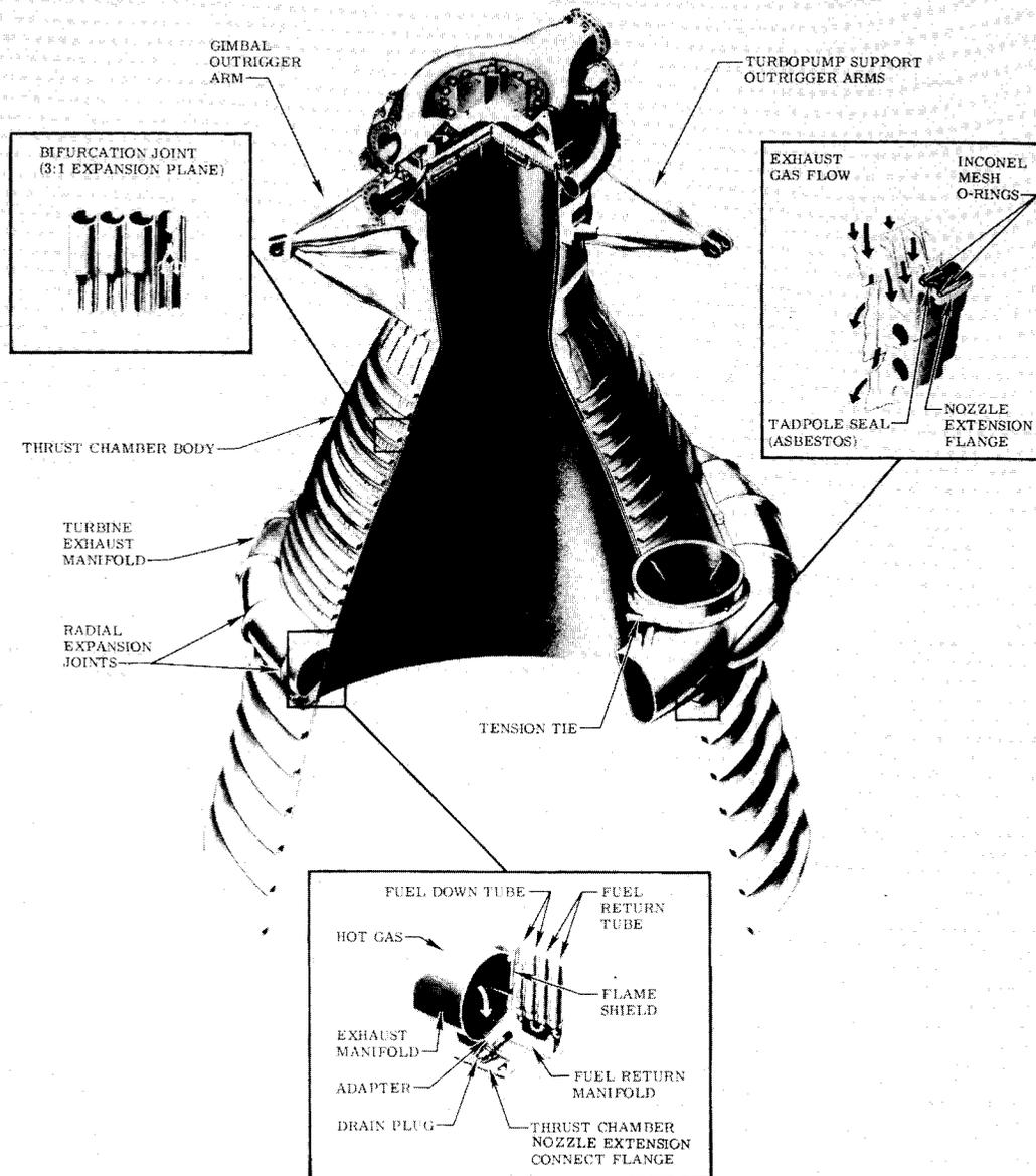
Fig. 2 Key features of the F-1 engine combustion chamber and injector body.
