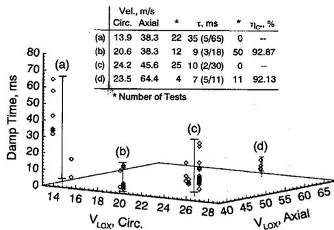
Fig. 11 Effect of oxidizer axial and circumferential injection velocities on damping characteristics and performance; unit 082,  $V_{RP-1} = 17.1$  m/s,  $(I.A.)_{RP-1} = 15$  deg.
