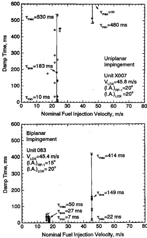
**Fig. 9 Damping characteristics exhibited by uniplanar (unit X007) and biplanar (unit 083) impingement injectors.**
