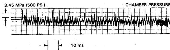
Fig. 5 Typical pressure-time trace exhibited during operation of injector units 005, 076, and 067.
