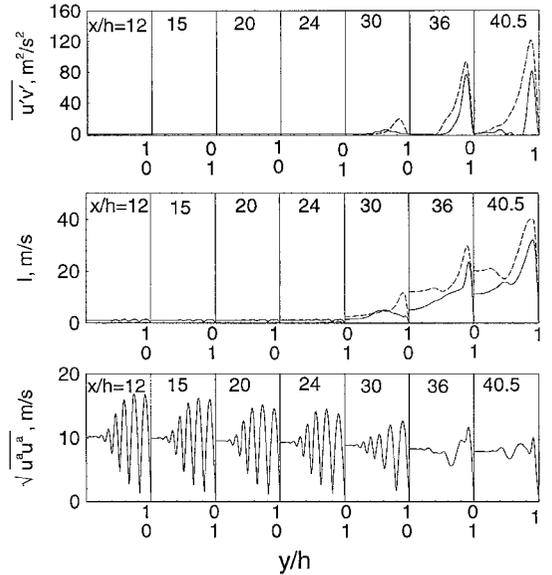
Fig. 12 Vertical distributions of Reynolds stress, turbulence intensity, and periodic-flow energy at various axial locations for  $f = 1800$  Hz and  $\epsilon = 5\%$ : ---, without forced oscillation and —, with forced oscillation.
