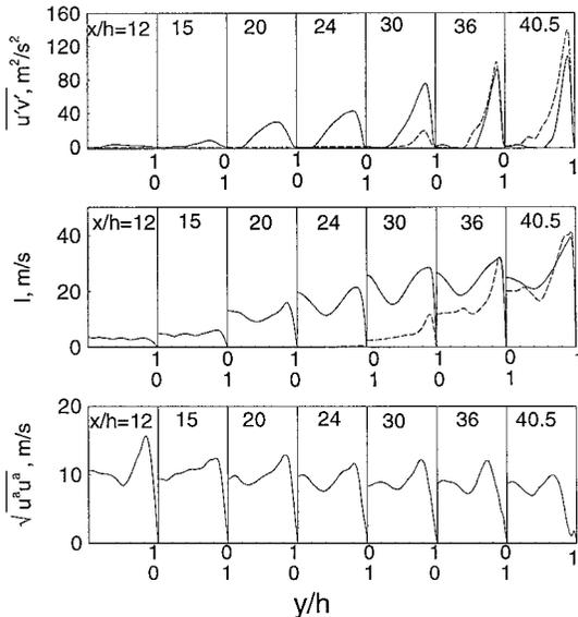
Fig. 11 Vertical distributions of Reynolds stress, turbulence intensity, and periodic-flow energy at various axial locations for  $f = 336$  Hz and  $\epsilon = 5\%$ : ---, without forced oscillation, and —, with forced oscillation.
