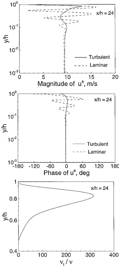
Fig. 16 Effect of turbulence on vertical variations of amplitude and phase of axial velocity fluctuation for  $f = 673$  Hz and  $\epsilon = 5\%$ ;  $x/h = 24$ .
