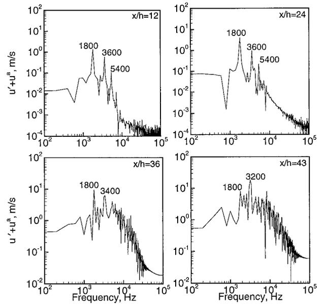
Fig. 9 Power spectral density of axial velocity fluctuations at various axial locations ( $f = 1800$  Hz and  $\varepsilon = 5\%$ );  $y/h = 0.9$ .
