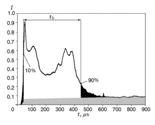
Fig. 13. Temporal variation of the intensity of light emitted by 80-nm aluminum particles in a gas consisting of CO<sub>2</sub> (50%) and N<sub>2</sub> (50%) at T = 1760 K and p = 32 atm [69]:  $t_b$  is the time period between 10 and 90% of the total integrated emission intensity; the background emission is marked by the gray color.
