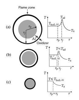
Fig. 15. Flame structures of aluminum particles in air: (a) micron-sized and larger particle (vapor-phase combustion); (b) micron-sized particles (combustion near the particle surface); (c) nanoparticles (surface combustion) [92].
