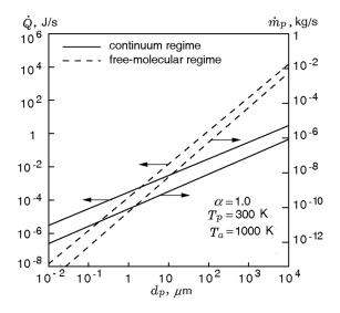
Fig. 4. Effect of the particle size on the heat transfer rate and the particle mass burning rate in the continuum and free-molecular regimes.
