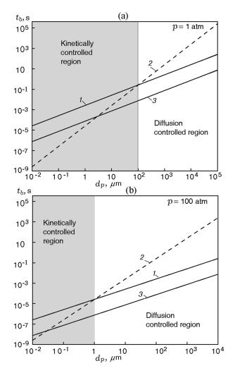
Fig. 6. Comparison of the aluminum particle burning times in air under diffusion-controlled and kinetically controlled conditions at pressures of 1 and 100 atm: curves 1 show the effect of chemical kinetics (at 3000 K); curves 2 and 3 show the effect of diffusion in the continuum (2) and free-molecular (3) regimes.
