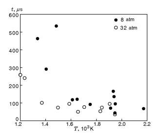
Fig. 20. Effect of pressure on the burning time of 80-nm aluminum particles in an oxygenated environment [69].
