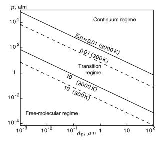
**Fig. 3.** Critical particle size for the transition from the continuum to the free-molecular regime as a function of pressure for two different temperatures: 300 and 3000 K.
