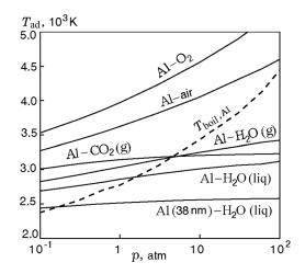
Fig. 9. Effect of pressure on the adiabatic flame temperature for different oxidizers and particle sizes.
