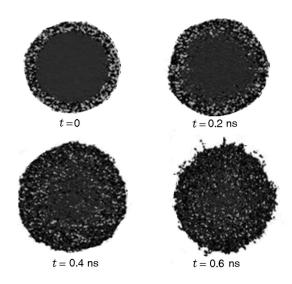
Fig. 8. Snapshots of the central slice of a 26-nm aluminum particle covered by an oxide  $(Al_2O_3)$  shell 3 nm thick: the images are obtained by means of molecular dynamics simulations; the snapshots show core Al atoms (black points), shell Al atoms (dark gray points), and shell O atoms (light gray points).
