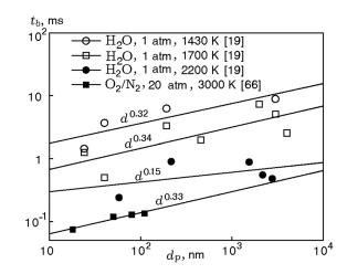
Fig. 17. Effect of the particle size on the burning time of nano aluminum particles with different oxidizers.
