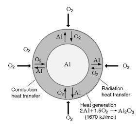
Fig. 5. Key physicochemical processes in combustion of nano aluminum particles in oxygen.
