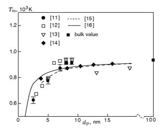
Fig. 1. Effect of the particle size on the melting temperature of nano aluminum particles [11].
