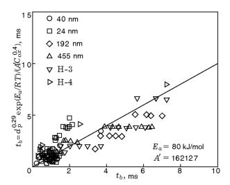
Fig. 19. Measured burning times of nano aluminum particles (points) versus the curve-fitting values (curve) ( $H_2O/Ar$ , 1 atm [19]).
