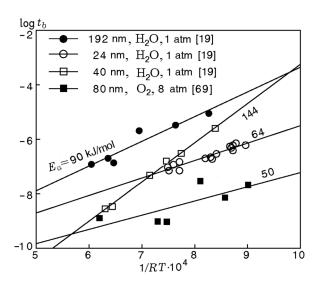
Fig. 16. Variation of the burning time of nano aluminum particles with the ambient gas temperature.
