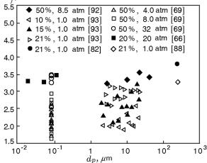
**Fig. 10.** Measured flame temperatures of aluminum particles as a function of the particle size for different pressures and oxygen concentrations.
