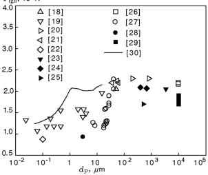
Fig. 2. Effect of the particle size on the ignition temperature of aluminum particles.
