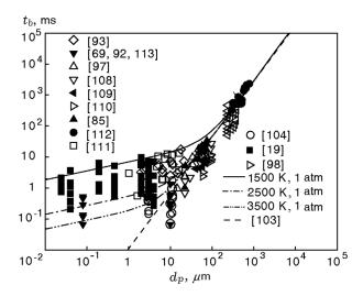
Fig. 21. Comparison of the burning time of aluminum particles obtained by using empirical correlations (curves) with experimental data (points).
