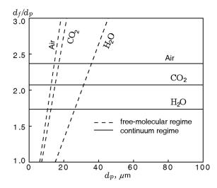
Fig. 14. Effect of the particle size on the maximum value of the flame-to-particle diameter ratio for different oxidizers [95].
