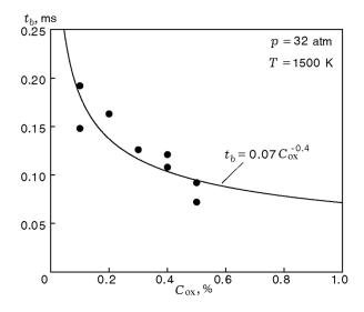
Fig. 18. Effect of the oxygen concentration on the burning time of 80-nm aluminum particles at p = 32 atm and T = 1500 K [69].
