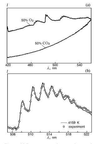
Fig. 12. (a) Emission spectra during combustion of 80-nm aluminum particles in oxygenated and carbon dioxide environments at p = 32 atm and T = 1900 K; (b) comparisons of the measured and fitted spectra for 80-nm particles in an oxygenated environment at T = 1600 K and p = 32 atm [69].
