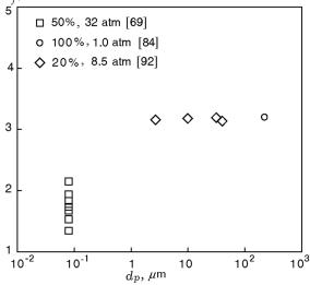
Fig. 11. Measured flame temperatures of aluminum particles as functions of the particle size for different pressures and carbon dioxide concentrations.
