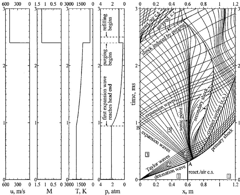
Fig. 8 First cycle  $x-t$  diagram and time histories of flow properties at head end under typical PDE operation: stoichiometric  $H_2$ /air mixture,  $\tau_{\text{cycle}} = 3$  ms,  $\tau_{\text{close}} = 2.4$  ms, and  $\tau_{\text{purge}} = 0.1$  ms; 1 = unburned region, 2 = Taylor expansion waves, 3 = stationary region, 4 = non-simple wave region, and 5 = simple wave region.
