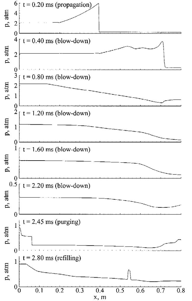
**Fig. 10** Time evolution of pressure distribution along centerline during first cycle of operation:  $\tau_{\text{cycle}} = 3$  ms,  $\tau_{\text{close}} = 2.4$  ms, and  $\tau_{\text{purge}} = 0.1$  ms.
