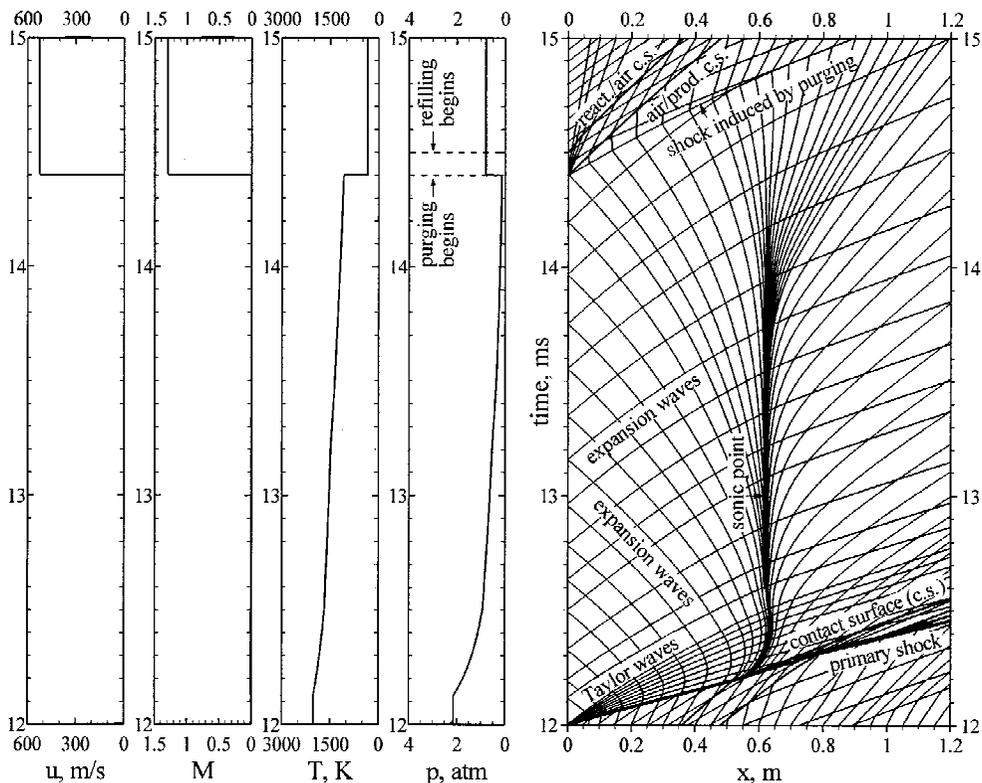
Fig. 11 Fifth cycle  $x-t$  diagram and time histories of flow properties at head end under typical PDE operation: stoichiometric  $H_2$ /air mixture,  $\tau_{cycle} = 3$  ms,  $\tau_{close} = 2.4$  ms, and  $\tau_{purge} = 0.1$  ms.
