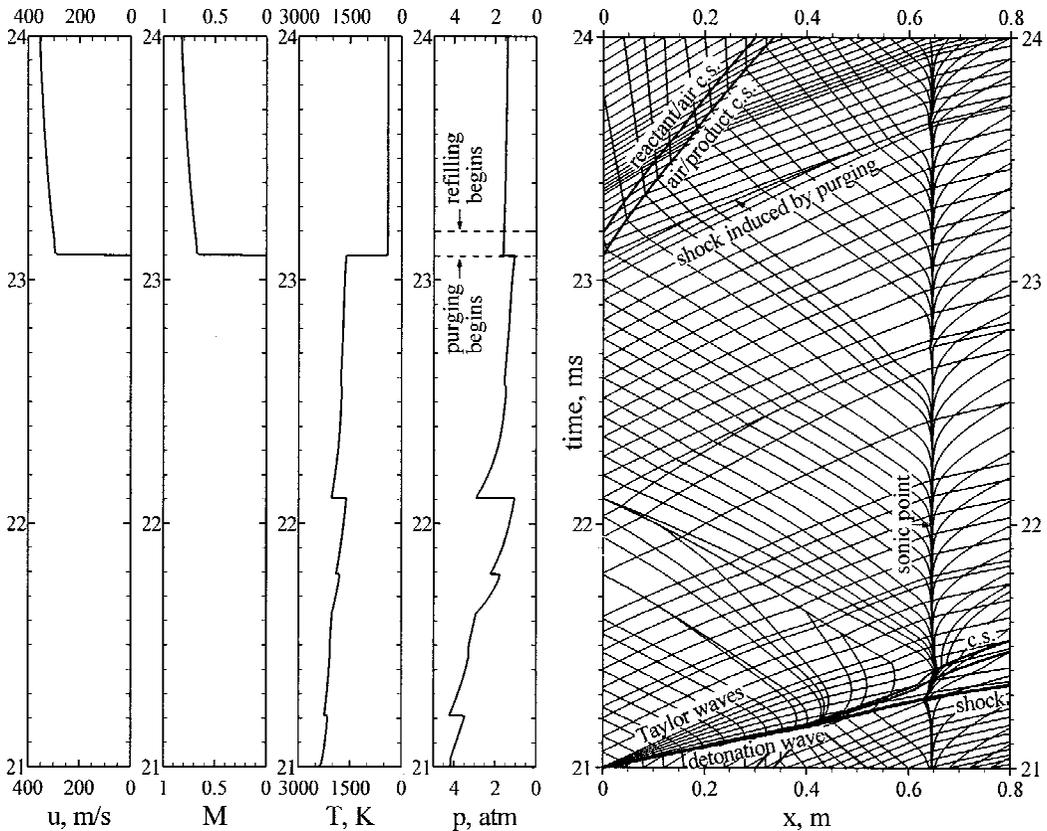
Fig. 15 Eighth cycle  $x-t$  diagram and time histories of flow properties at head end under typical PDE operation with C-D nozzle: stoichiometric  $H_2$ /air mixture,  $\tau_{\text{cycle}} = 3$  ms,  $\tau_{\text{close}} = 2.1$  ms, and  $\tau_{\text{purge}} = 0.1$  ms.
