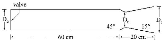
Fig. 13 Configuration of single-tube PDE with C-D nozzle.
