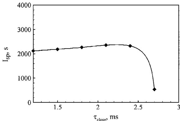
Fig. 12 Effect of valve close-up time on specific impulse,  $\tau_{cycle} = 3$  ms and  $\tau_{purge} = 0.1$  ms; straight tube with stoichiometric  $H_2$ /air mixture,  $h = 9.3$  km, and  $M_\infty = 2.1$ .
