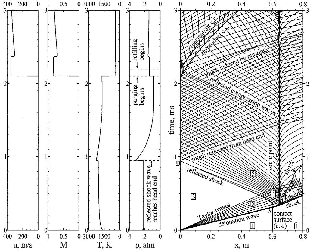
Fig. 14 First cycle  $x-t$  diagram and time histories of flow properties at head end under typical PDE operation with C-D nozzle: stoichiometric  $H_2$ /air mixture,  $\tau_{\text{cycle}} = 3$  ms,  $\tau_{\text{close}} = 2.1$  ms, and  $\tau_{\text{purge}} = 0.1$  ms; 1 = uniform unburned region, 2 = Taylor expansion waves, 3 = uniform region, 4 = non-simple wave region, and 5 = simple wave region.
