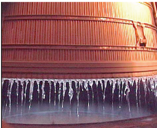
Fig. 7 CECE at 30% power levels showing ice formation [39,40].
