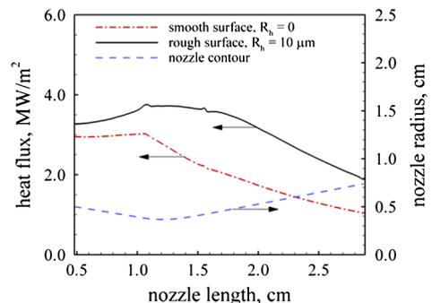
**Fig. 4 Comparison of heat-flux to nozzle surface for smooth and rough surfaces; no radiation.**
