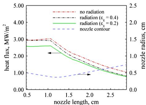
Fig. 6 Comparison of heat-flux to nozzle surface for cases with and without radiation; smooth surface.
