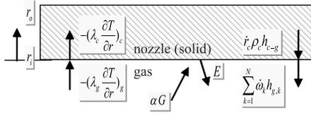
**Fig. 1 Schematic of energy balance at gas-solid interface with radiation.**
