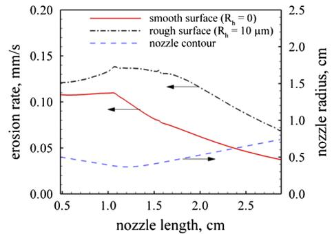
**Fig. 3 Comparison of nozzle erosion rate for smooth and rough surfaces; no radiation.**
