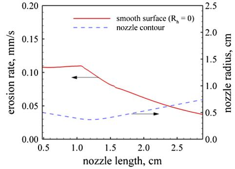
**Fig. 2 Baseline nozzle erosion rate for smooth surface without radiation.**
