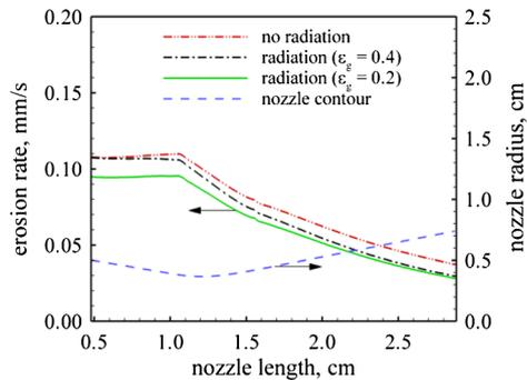
Fig. 5 Comparison of nozzle erosion rate for cases with and without radiation; smooth surface.
