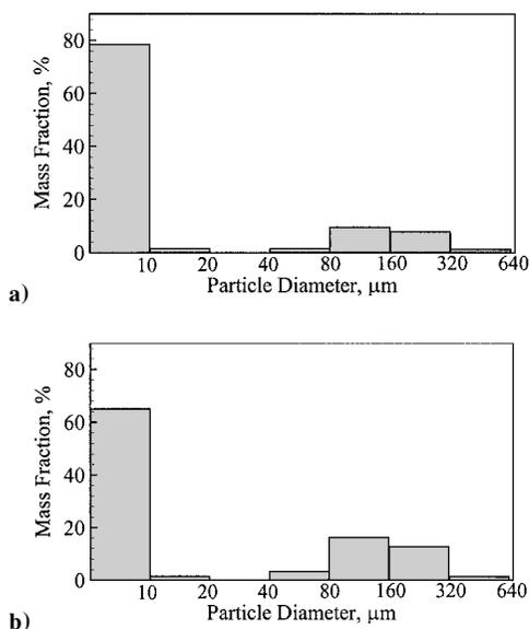
**Fig. 15** Particle size distribution in laminar flow with first longitudinal mode of acoustic oscillation ( $f = 1885$  Hz,  $C_m = 0.2$ , and  $\varepsilon = 0.02$ ) at a) injection surface and b) chamber exit.
