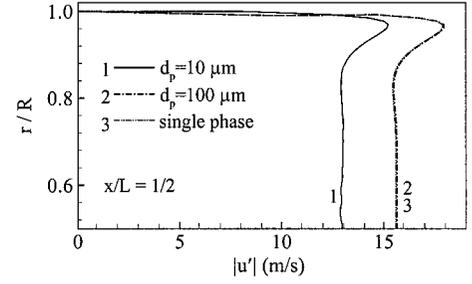
**Fig. 12** Amplitude of axial velocity fluctuation in turbulent flow with first longitudinal mode of acoustic oscillation ( $f = 3770$  Hz,  $C_m = 0.2$ , and  $\varepsilon = 0.02$ ) at  $x/L = \frac{1}{2}$ .
