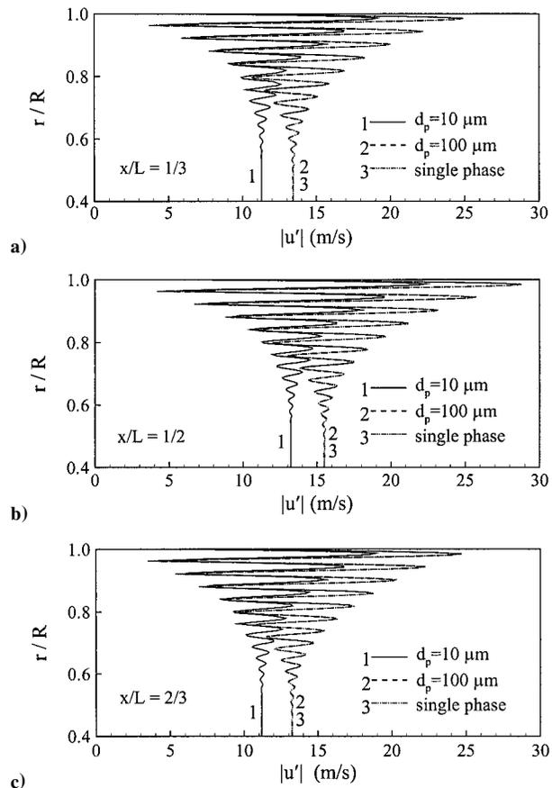
Fig. 10 Amplitudes of axial velocity fluctuation in laminar flow with first longitudinal mode of acoustic oscillation ( $f = 1885 \text{ Hz}$ ,  $C_m = 0.2$ , and  $\varepsilon = 0.02$ ) at a)  $x/L = \frac{1}{3}$ , b)  $x/L = \frac{1}{2}$ , and c)  $x/L = \frac{2}{3}$ .
