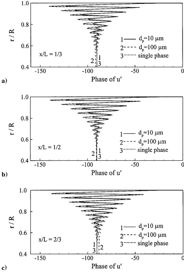
**Fig. 11** Phases of axial velocity fluctuation in laminar flow with first longitudinal mode of acoustic oscillation ( $f = 1885$  Hz,  $C_m = 0.2$ , and  $\varepsilon = 0.02$ ) at a)  $x/L = \frac{1}{3}$ , b)  $x/L = \frac{1}{2}$ , and c)  $x/L = \frac{2}{3}$ .
