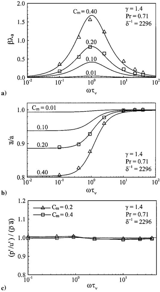
**Fig. 2** Effect of particles on a) attenuation, b) dispersion, and c) impedance of acoustic waves in two-phase mixtures:  $\triangle$  and  $\square$ , numerical simulation, and —, theoretical prediction.
