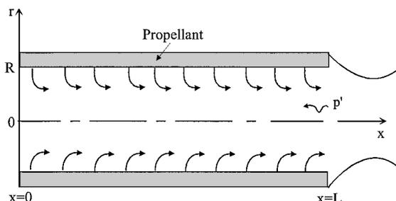
Fig. 1 Schematic diagram of a solid rocket motor.
