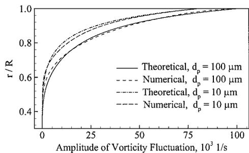
**Fig. 14** Comparison between analytical and numerical solutions of amplitude of vorticity fluctuation in laminar flow with first longitudinal mode of acoustic oscillation ( $f = 1885$  Hz,  $C_m = 0.2$ , and  $\varepsilon = 0.02$ ) at  $x/L = \frac{1}{2}$ .
