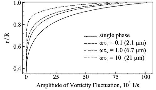
**Fig. 13** Analytical solution of amplitude of vorticity fluctuation in laminar flow with first longitudinal mode of acoustic oscillation ( $f = 1885$  Hz,  $C_m = 0.2$ , and  $\varepsilon = 0.02$ ) at  $x/L = \frac{1}{2}$ .
