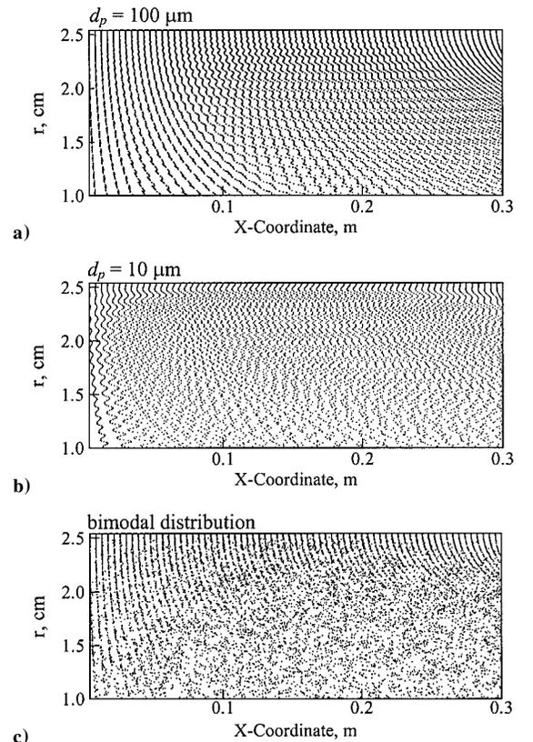
**Fig. 8** Snapshots of particle field in laminar flow with first longitudinal mode of acoustic oscillation ( $f = 1885$  Hz): a)  $d_p = 100 \mu\text{m}$ , b)  $d_p = 10 \mu\text{m}$ , and c) bimodal size distribution.
