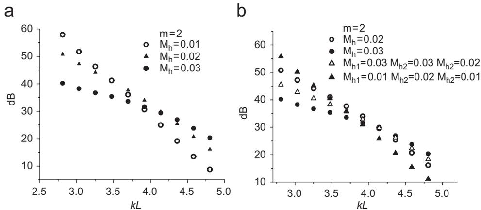
Fig. 8. Effect of the variations of frequency and bias flow on the attenuation.
