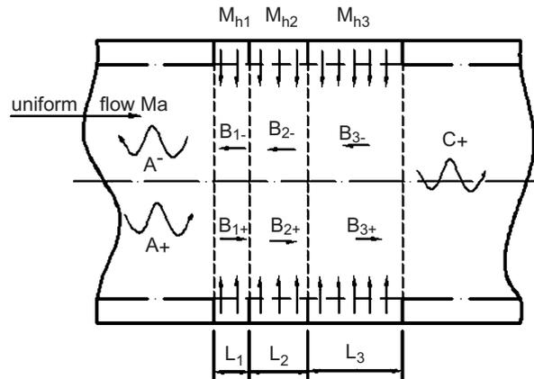
Fig. 7. The geometry of segmented non-locally reacting liners,  $L_1 = 0.15\text{ m}$ ,  $L_2 = 0.25\text{ m}$ ,  $L_3 = 0.40\text{ m}$ ,  $a = 2\text{ mm}$ ,  $r_1 = 1.0\text{ m}$ ,  $r_2 = 1.2\text{ m}$ ,  $\phi = 4\%$ .
