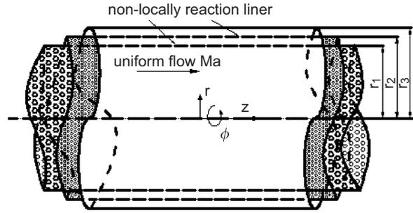
Fig. 5. A circular duct with double-layer, acoustically non-locally reacting liner circular duct.
