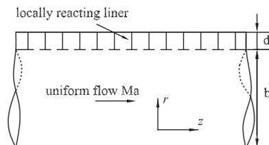
Fig. 1. The geometry of an acoustically locally reacting liner two-dimensional duct.
