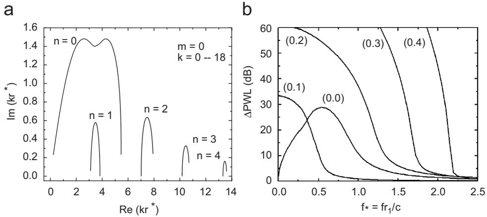
Fig. 4. Effect of frequency variation on the eigenvalues (a) and insertion loss (b),  $r_1 = 1.0\text{ m}$ ,  $h = 0.2$ ,  $Ma = 0$ ,  $L = 1.0$ ,  $a = 3\text{ mm}$ ,  $\phi = 5\%$ ,  $Ma(U) = U/c_0 = 0.03$ .
