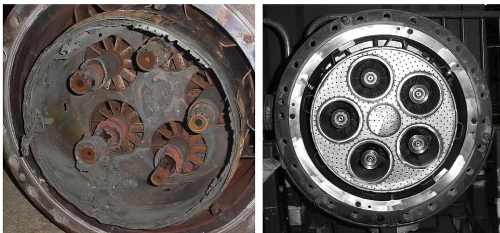
Fig. 1. Burner assembly (left) damaged by combustion instability and new burner assembly (right) (Goy et al. [7]).
